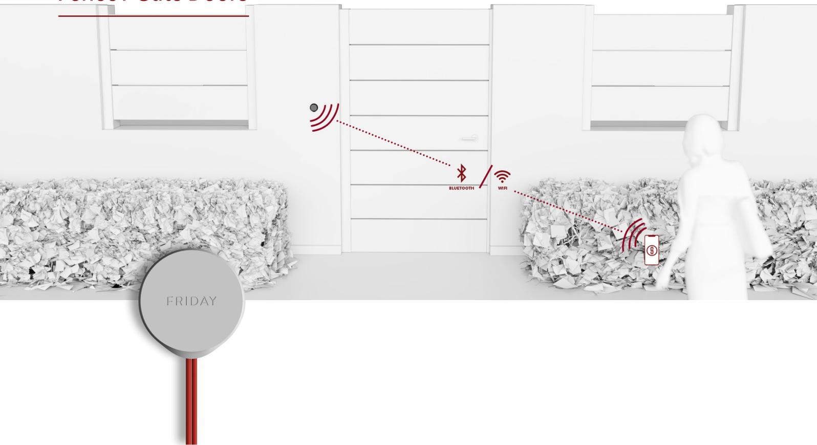
New smarter access to your existing or new electrical installations. Install LINK in the electrical installation who supply power to the electrical Strike, door automation or electromagnetic lock. Open and close doors with the FRIDAY app through Bluetooth or Wi-Fi. Remote open and close doors through FRIDAY Access.
