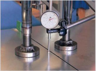
To determine the point load, a static load (such as a table leg) is simulated. On the basis of the permissible point load thus established, the system is generally assigned an appropriate load and deflection class. In accordance with standard practice, the load is applied with a 25 mm x 25 mm indentor.
