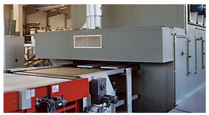
Our modern powder-coating facility; spare powder that has not been applied onto the work piece is always re-circulated into the coating process without any forfeit of quality for the end product.
