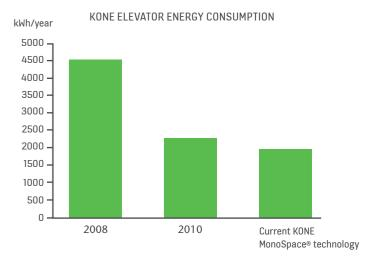
The calculation is based on an elevator speed of 1 m/s, a load of 1600 kg, 200,000 starts/year, a travel height of 16 m and 5 floors
