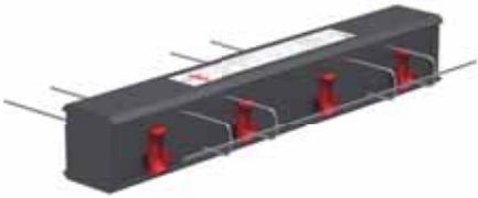
Figure: Type HIT-SP ZVX-0404...-06 Bent bar type; shear bars \phi 6 mm (also available for custom designs in \phi 8 mm)
