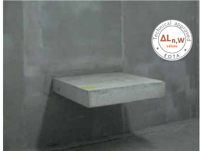
Test setup according to EN ISO 10140 with built-in element
