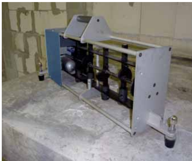
Standardised tapping machine according to EN ISO 10140
