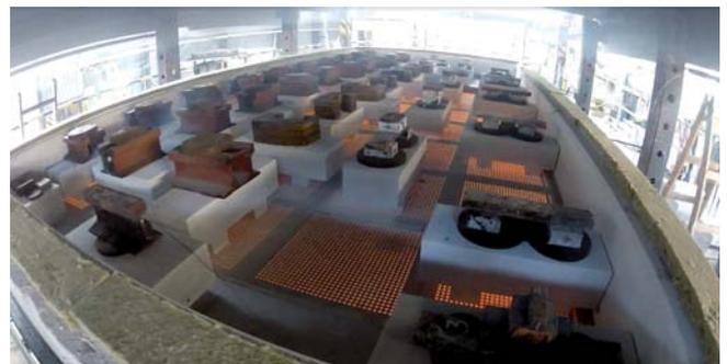
Lindner FLOOR and more® is suited for the use in these areas due to its reaction to fire performance A1 according to EN 13501-1. The system has the respective F 30-AB / REI 30 classifications according to DIN 4102-4 respectively EN 13501-2.
