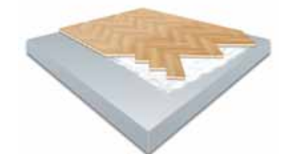
Patterned parquet, MS-Polymer adhesive, layer of concrete
