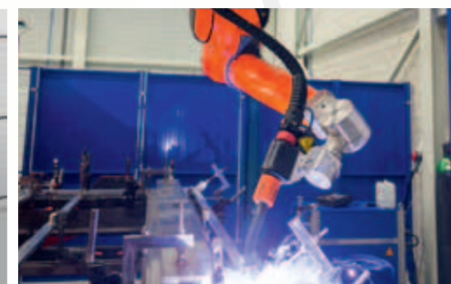
Welding Steel sheet panels protect from sparks, dust, liquids and welding light.
