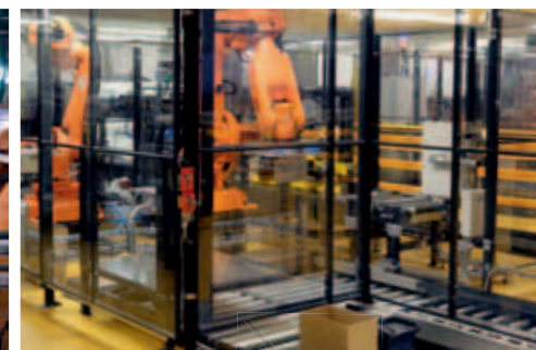
Production Line The ST PC polycarbonate panels give good visibility.
